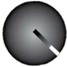
Turning the OTL all the way to the right (clockwise) prevents the heating cutoff system from interfering with this procedure.
