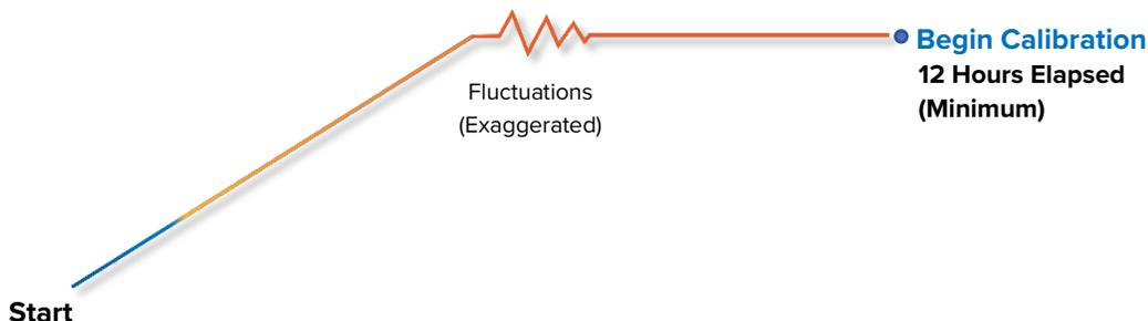
Required temperature stability period operating undisturbed with the incubator
