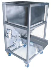
FM-212 feeder machine with custom rectangular supply hopper.
