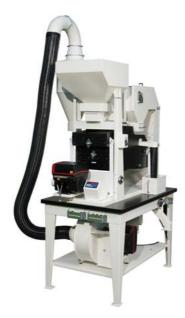
The LA-LS air/screen cleaner is a precision and fine cleaner for laboratory use as well as for small-scale production in research stations, institutes etc.
