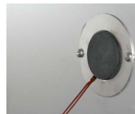
Figure 19: Introducing a sensor probe through the access port.
