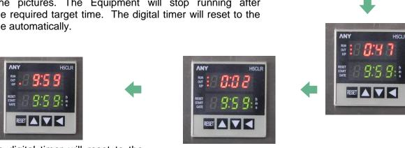
7. The digital timer will reset to the last target time automatically.
