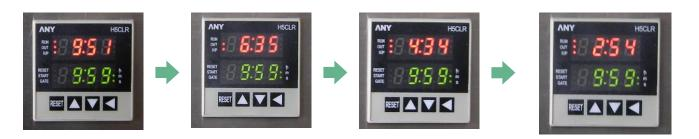
6. While the test is in progress, the timer is counting down the time as shown on the pictures. The Equipment will stop running after completing the required target time. The digital timer will reset to the last target time automatically.
