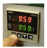
**4.** Press the RST KEY <u>to</u> save the new desired target
