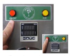
**1.** Turn the equipment on by pressing - the ON-OFF Red Push Button -
