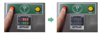
8. To turn the Seed Blower OFF, press the Red Push Button. This Button is also used to STOP the equipment in case of an emergency. Also Read Note B.
