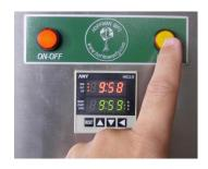
**5.** Press the Amber Push Button (as shown) to run the test. The timer will countdown
