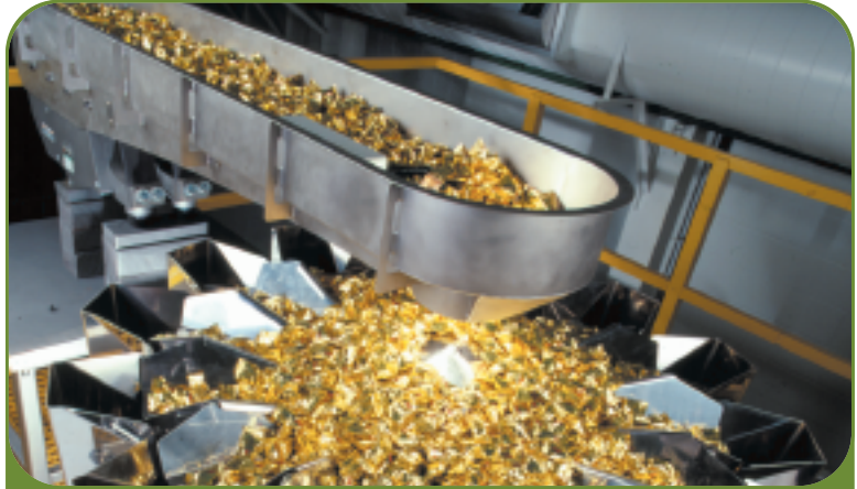
Syntron BF-4 Feeder with peripheral discharge feeds candy to a weigh scale.
