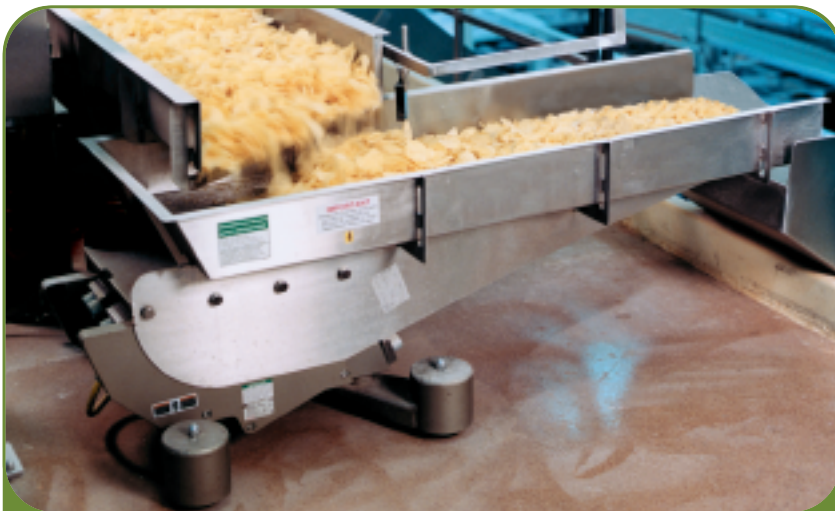
The Syntron BF-4 Low Frequency Feeder features coil spring isolation.
