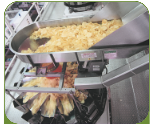
Syntron Model BF-2 Feeders feed potato chips from a modular distribution system to weigh scales in a typical snack food packaging application.
