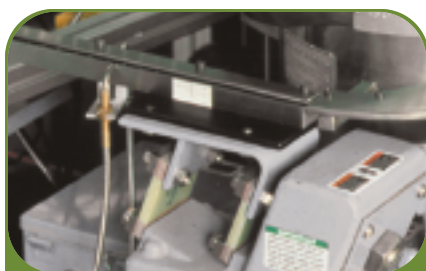
Syntron vibra drives are used by many different industries. Here, an F-T01 drive in a parts handling application.
